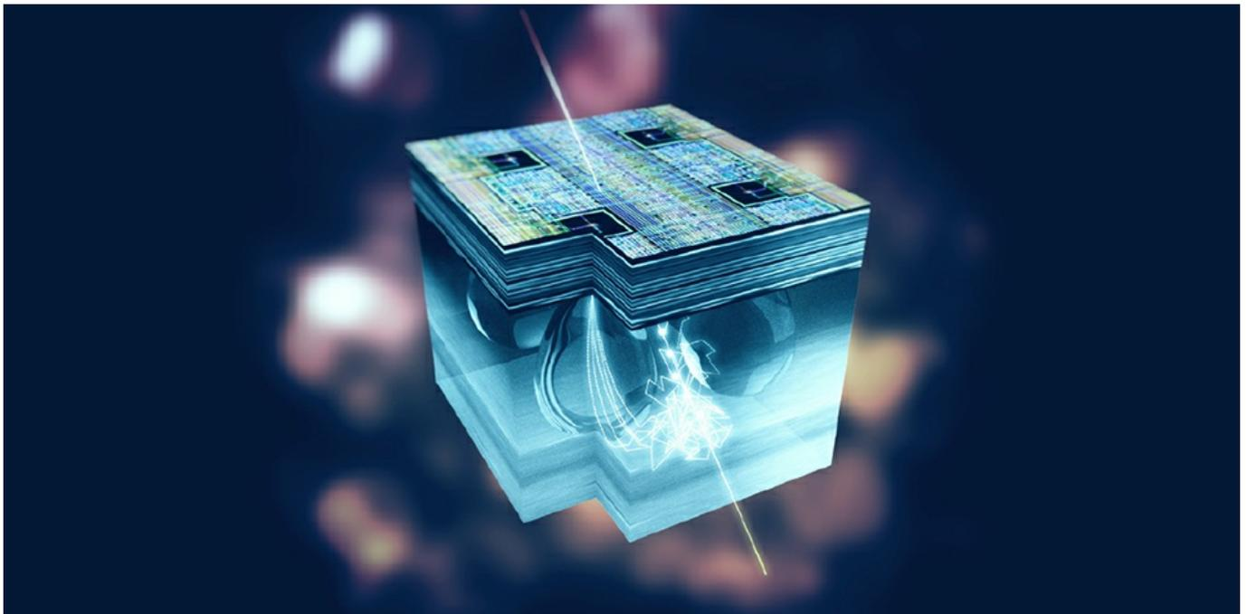
Illustration of microelectronics circuitry integrated with a detecting medium as a single monolithic solid-state detector. Credit: © ALICE collaboration.
