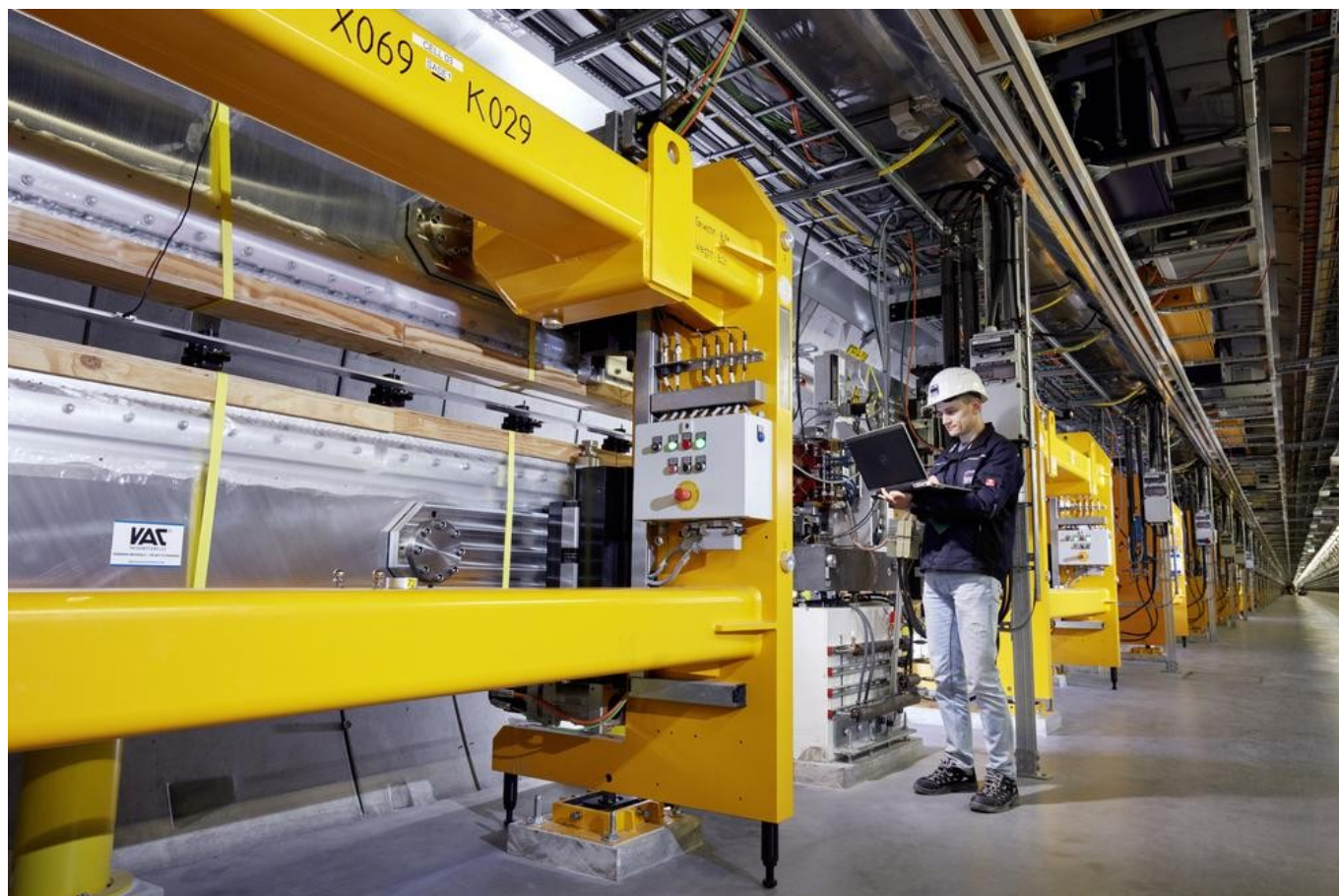
I magneti "ondulatori" usati per produrre la radiazione X. / The undulators used to generate the X-ray radiation. Credits: European XFEL/Heiner Müller-Elsner
